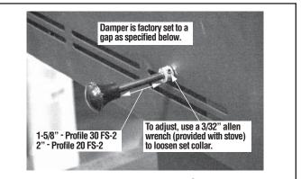
Figure 10 - Damper Adjustment, Free-Standing Models
